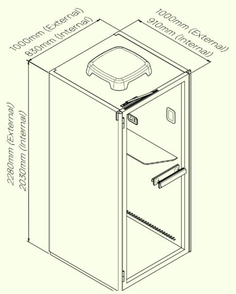
Each Mello POD contains as standard, laminate hard wearing table surface. Power Consumption for MELLO, 0.18A.
